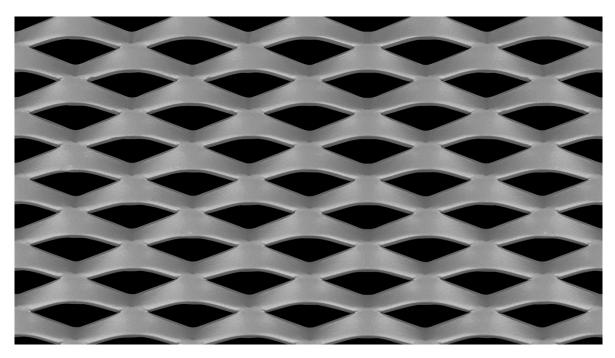
LW Pitch:30.48mmStrand Width:6.00mmSW Pitch:17.50mmThickness:2.00mmWeight:3.70 kg / m2Open Area:31%
